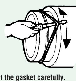
Fit the gasket carefully. Equalize the rubber gasket stretch by running a smooth, round object, inserted between gasket and spigot, around the entire circumference several times.
