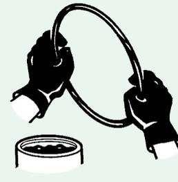
Lubricate the gasket thoroughly before it is placed on the spigot or tongue.
