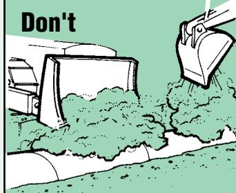
Backfill material should be bulldozed into the trench or dropped directly on the pipe. Material should be placed in such a manner so as not to displace or damage the installed pipe.
